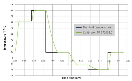
Detailed image from step test: Fast settling to ±0.005 °C.
